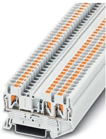
Feed-through terminal block, nom. voltage: 800 V, nominal current: 24 A, connection method: Push-in connection, 1 level, Rated cross section: 2.5 mm<sup>2</sup>, cross section: 0.14 mm<sup>2</sup> - 4 mm<sup>2</sup>, mounting type: NS 35/7,5, NS 35/15, color: white
